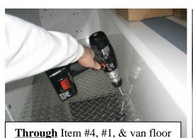
Attach to wood floor or rubber floor mat using #10 x 1" Phillips pan head sheet metal screws
